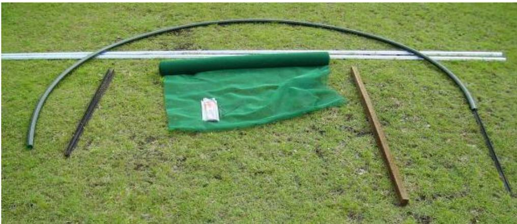
Photo3, materials. Top: ceiling battens. L to R: poly-pipe arch; star picket; tie-wires on shade-cloth; upright. Not on photo: door; hinges; latch; metal strapping.
